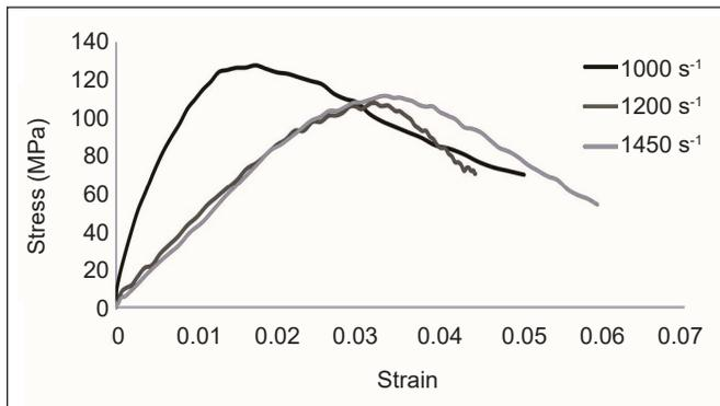
Figure 9. Compressive stress-strain curve of kenaf composite under different strain rates
