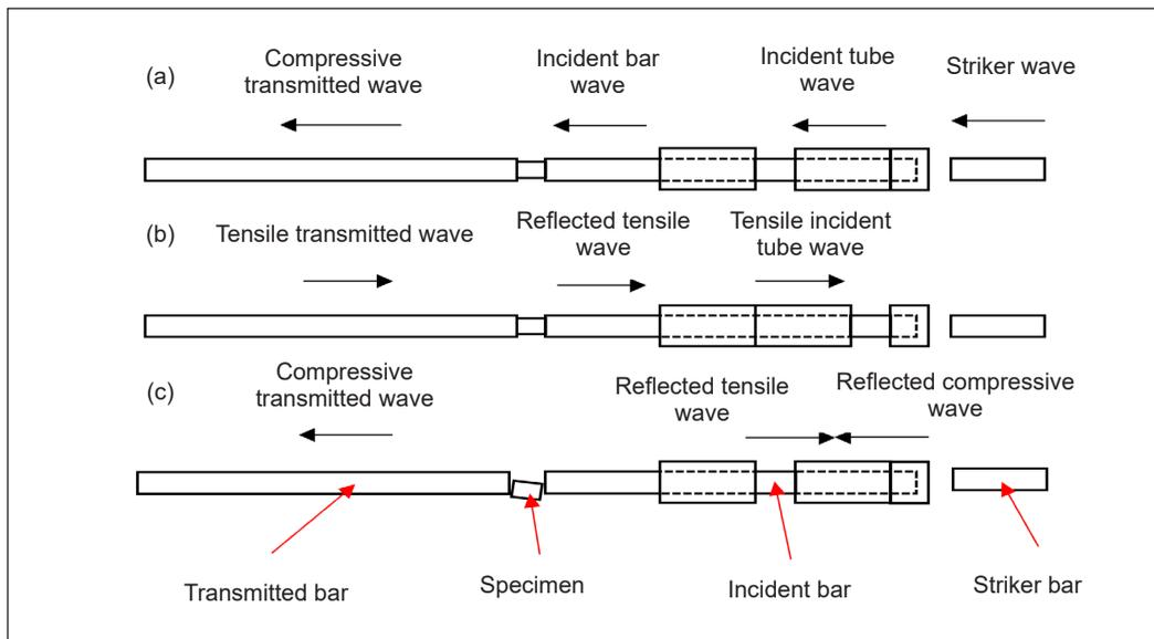
Figure 3. Schematic illustration of the operating principle of a standard SHPB with a momentum trap
