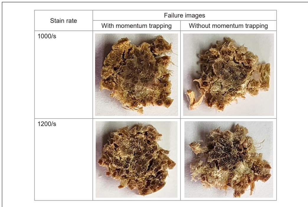
Figure 10. Failures of kenaf composite under different strain rates with and without momentum trapping
