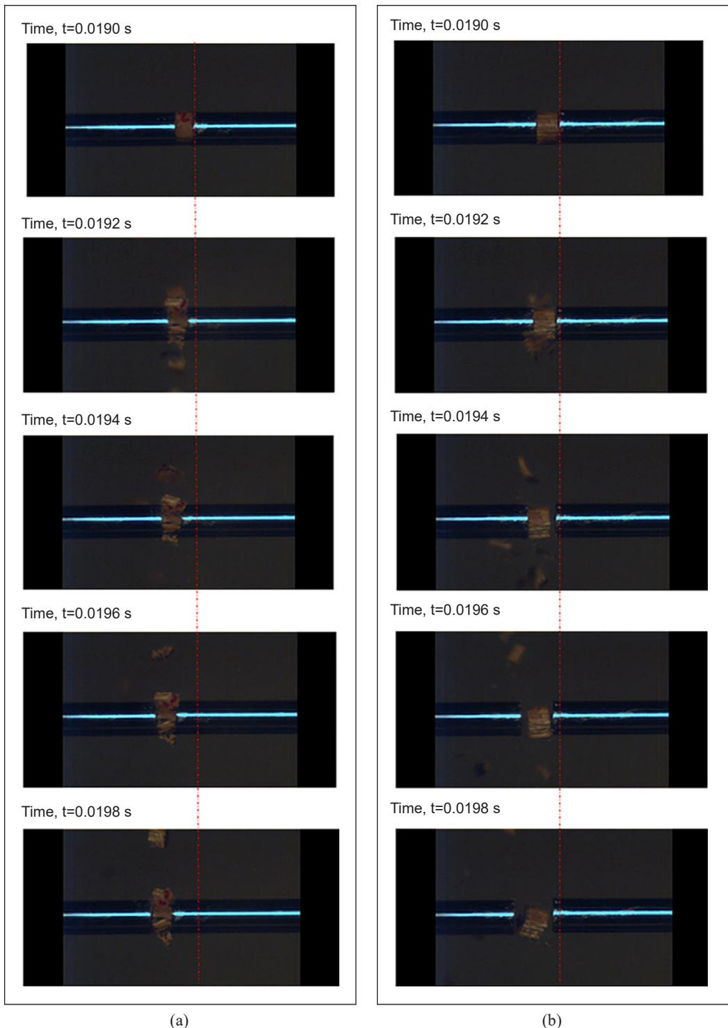
Figure 7. High speed images of specimen's condition during impact loading (a) without momentum trap (b) with momentum trap
