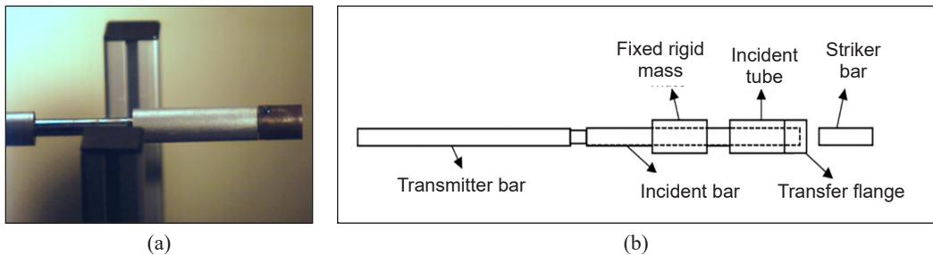
Figure 2. (a) Implementation of a momentum trapping on a SHPB; and (b) Schematic illustration of momentum trapping on a SHPB
