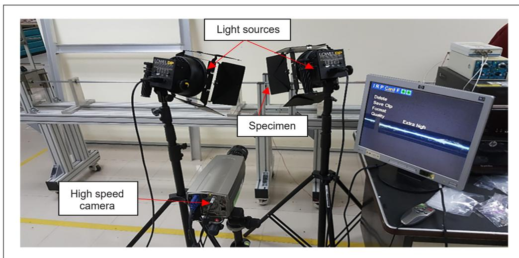
Figure 4. High speed camera setup during impact loading
